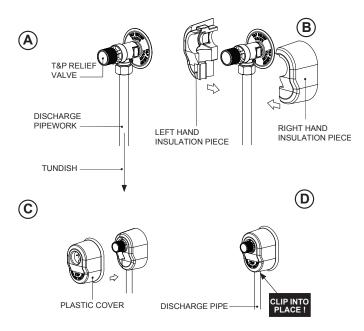
Figure 10: T&P Relief Valve insulation set installation
