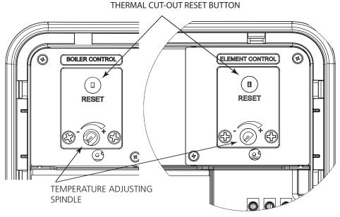
Figure 14: Thermostat adjustment
