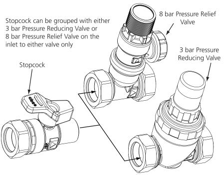
Figure 8: Cold water controls - installation combinations
