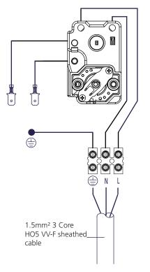
Figure 13: Wiring schematic - DIRECT models
