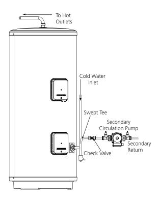
Figure 9: Secondary circulation schematic
