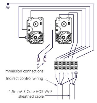
Figure 15: Wiring schematic - INDIRECT models
