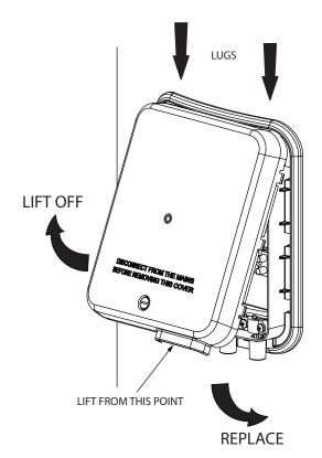
Figure 12: Immersion heater cover removal and replacement
