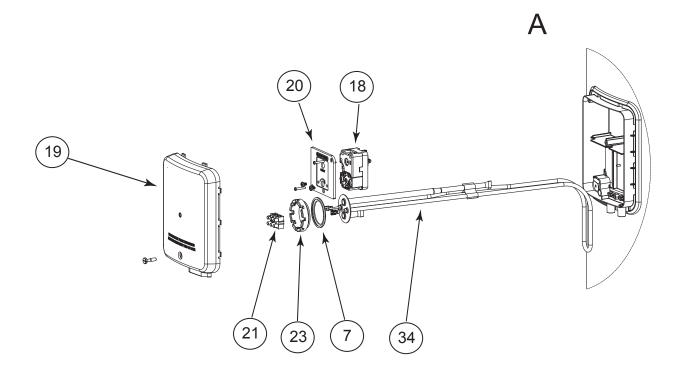
Spare components are common to Upper and Lower Direct Control Assemblies except for the Upper element 34 and Lower element 16
