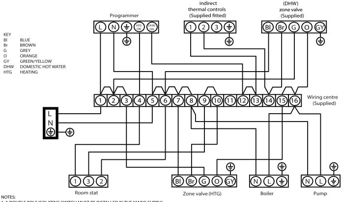
1. A DOUBLE POLE ISOLATING SWITCH MUST BE INSTALLED IN THE MAINS SUPPLY. 2. ALL EARTH CONNECTIONS MUST BE LINKED BACK TO THE MAINS EARTH SUPPLY.
