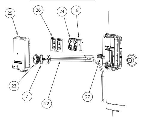
Figure 20: Indirect controls and immersion heater, exploded view
